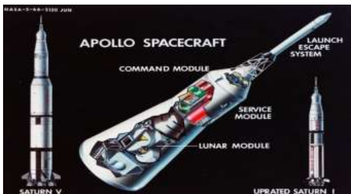
Fig. 3. The Apollo payload: the command module, the service module and the lunar module.
